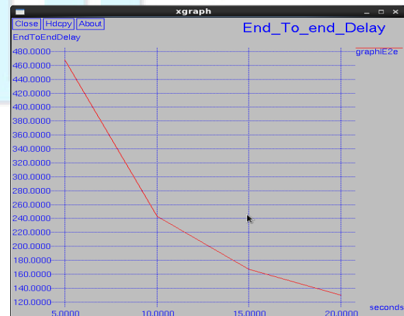
Fig. 4 End to end delay in attack detection
